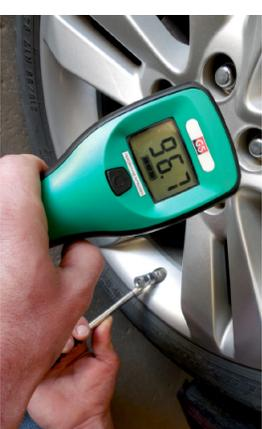
Shawn Pease, TIA director of automotive tire service, notes, "TPMS tool manufacturers are routinely releasing software updates throughout the year. Many factors can initiate a software change, such as new sensor technologies, vehicle model introductions or vehicle recalls. Keeping the TPMS tool software up to date helps ensure faster, more successful TPMS service with fewer comebacks."
