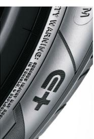
Yokohama Rubber Co. photo. Yokohama is marking tires built for electric vehicles with a proprietary "E+" mark on the sidewall to distinguish them from other tires in the same line.
