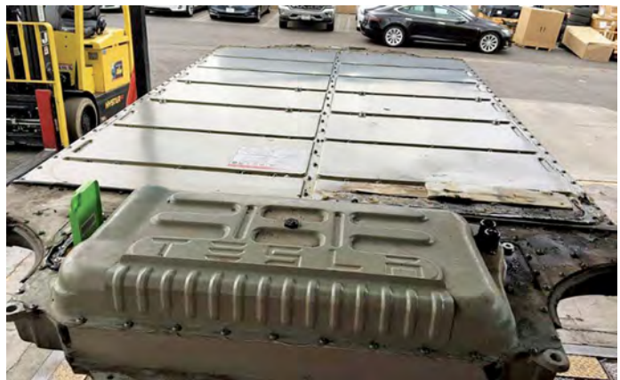
Battery case from a Tesla Model S after a noncrash-related fire in West Hollywood, Calif., in 2018
