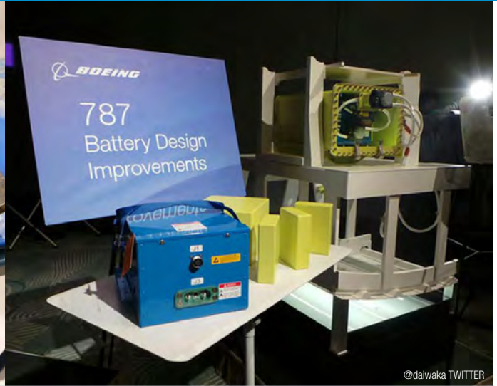
The exterior case of a thermal-damaged lithium ion battery that caught fire in a Japan Airlines' 787 in 2013 (left) and the redesigned battery (right).
