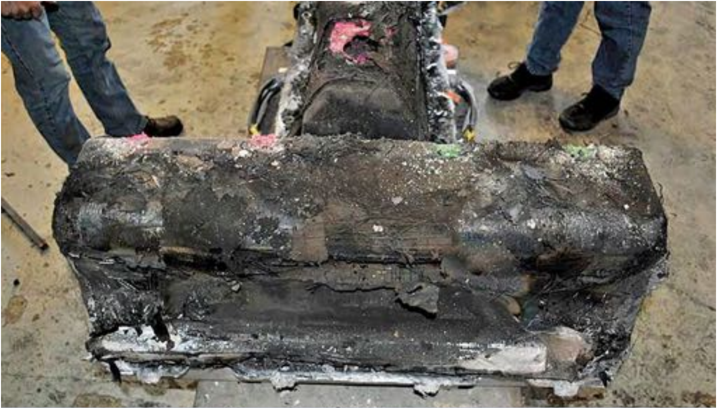
Chevy Volt battery damaged in a 2011 fire that erupted three weeks after a crash test
