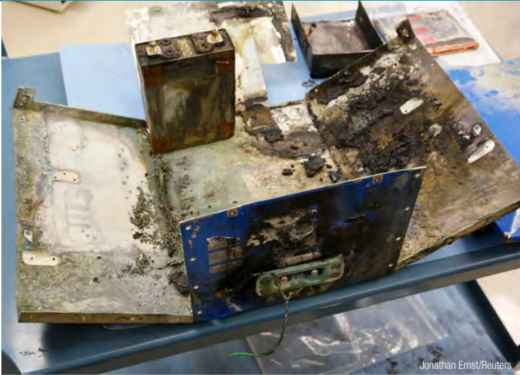
The exterior case of a thermal-damaged lithium ion battery that caught fire in a Japan Airlines' 787 in 2013 (left) and the redesigned battery (right).
