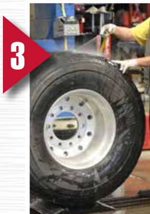
3 SPRAY TIRE DOWN ON ROLLER BASE
